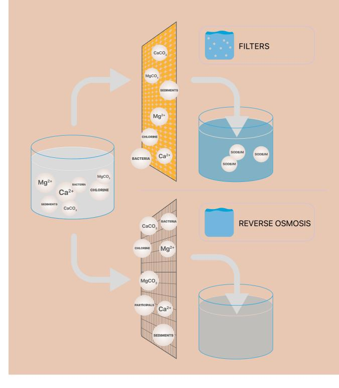
Filters allow the mains water supply to be purified of all those substances that alter its taste and smell, or which compromise its drinkability. To control its taste and smell, activated carbon is used, such as the Carbon Block Profine<sup>®</sup>, which intercepts any particulate matter and chlorine thanks to its properties of absorption. On the other handf, or toxic substances such as pfas, nitrates and arsenic, specially designed filters are used. **Reverse osmosis**
